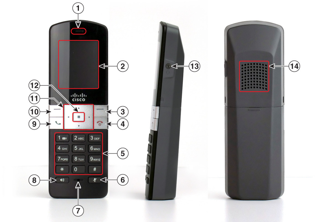
Figure 1 Cisco SPA302D Mobility Enhanced Cordless Handset Phone Components
